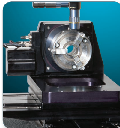
Phi motorized rotation stage (with variable chuck to hold parts) mounted on top of motorized X, Y stage.
