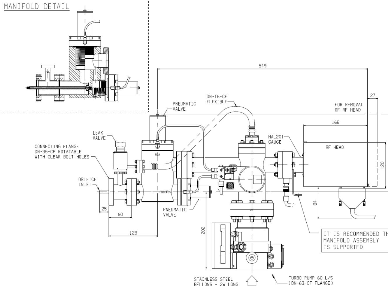
The leak valve option shown extends the sampling pressure range.
