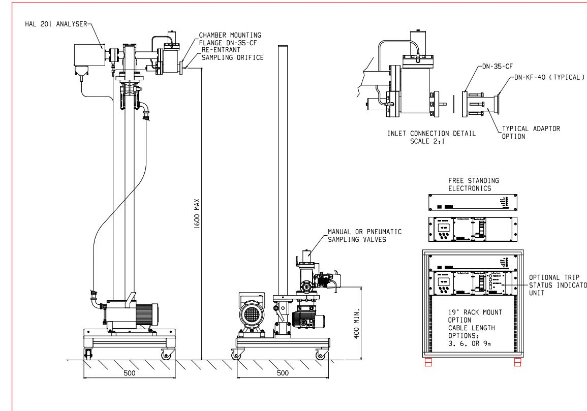
The cart mounted design has a small footprint, adjustable height, and is easily moved from process tool to tool.
