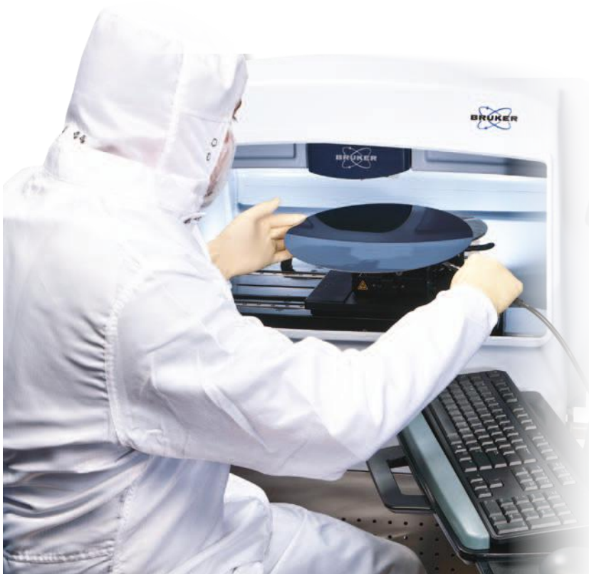
Operator loading 300mm wafer onto Dektak XTL.
