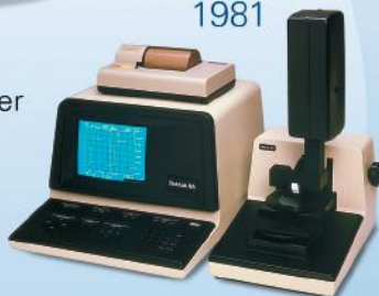
Dektak IIA First Micro-Processor Based Profiler
